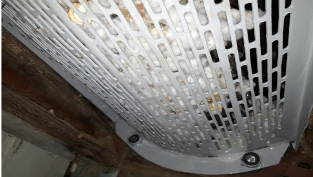
Figure 3. A prototype of a multifaceted grid surface mounted on the UGC cotton ginning unit.
