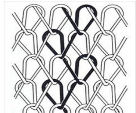
Fig. 2. Basic pattern of warp knitting
