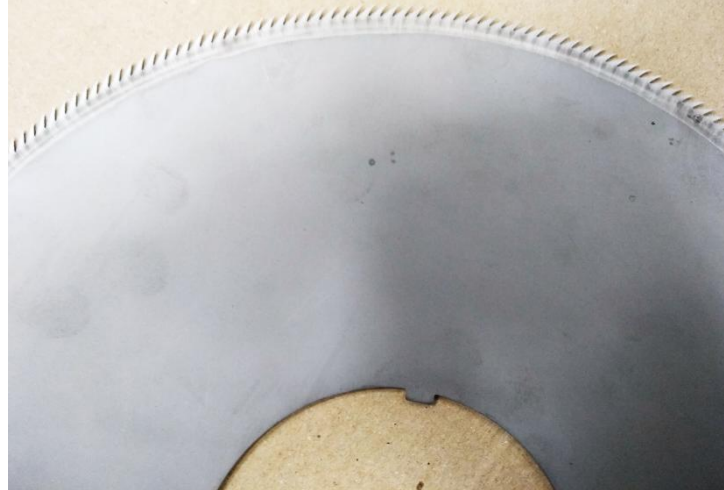
Fig. 4. Circular saw after nitriding.
