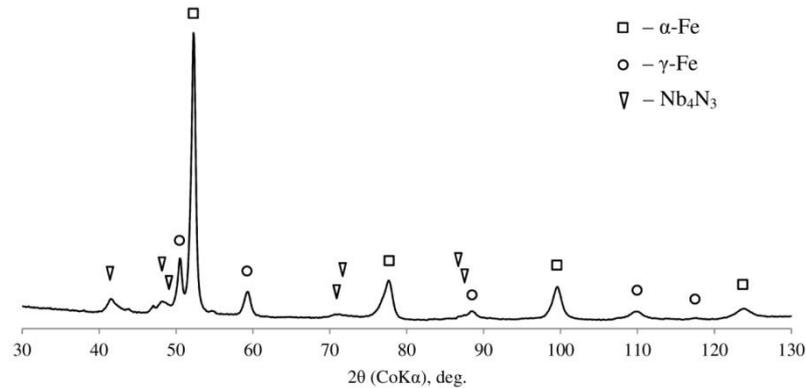
**Fig.5** Diffraction pattern (CoKα) from the surface of the sample of nitrided steel R6M5 after coating the surface of the film of NbHfTi alloy before irradiation
