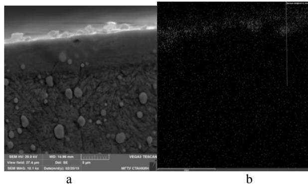
**Fig.4.** The surface layer of high-speed steel P6M5 modified by zirconium nitride. a) SEM image of pickled section, b) zirconium distribution map of section.
