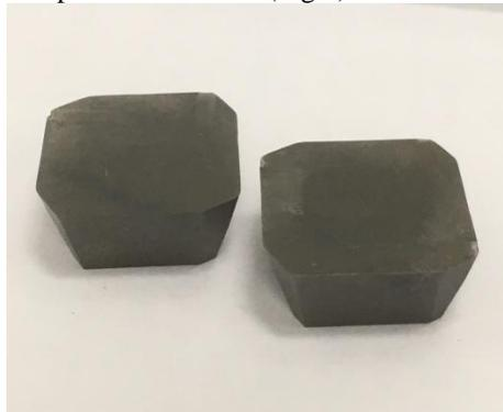
**Fig.1.** Strengthened cutting plates from steel R6M5 (M2).
