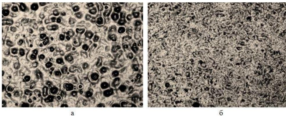
**Fig.2** a) Structure of the surface of nitrated high-speed steel R6M5 after exposure to NESP, b) Same after electron-beam alloying with zirconium.
