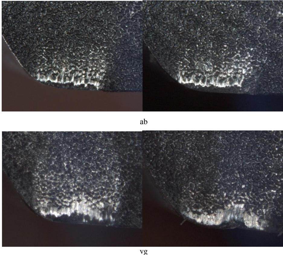
**Fig.9.** Wear plate of steel R6M5 (nitriding + micro alloying alloy  $Nb_{70}Hf_{22}Ti_8$  + coating) when turning alloy heat-resistant steel,  $v = 10\text{m/min}$ ,  $s = 0.115\text{ mm/rev}$ ,  $t=1\text{mm}$ , a) after 6 min., b) after 10 min. v) after 15 min. g) after 21 min of cutting.
