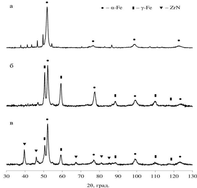
**Fig.3.** a) A diffractogram (CoC $\alpha$ ) from the surface of a sample of nitrated steel R6M5, b) the same after exposure to NESP, c) the same after deposition of Zr film on the surface before irradiation.
