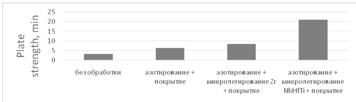
**Fig.6** Durability of plates with a combined surface treatment (min).
