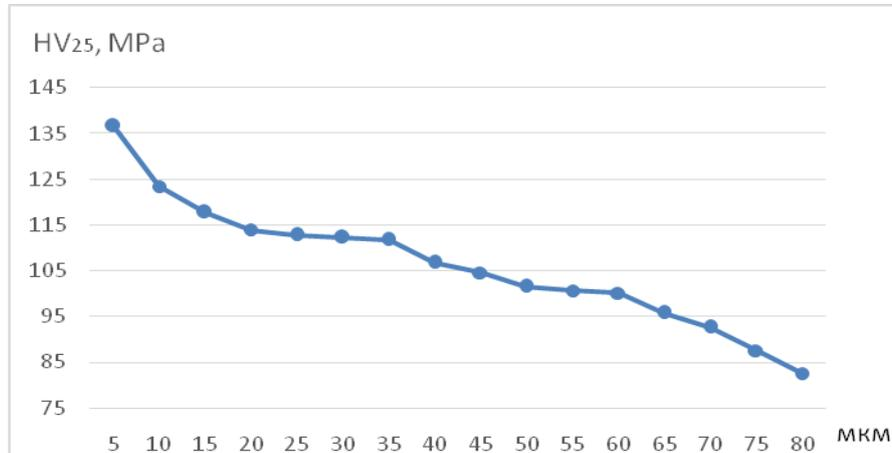
**Fig.6.** Change of micro hardness over the depth of the hardened zone on the transverse section with a sample of steel R6M5 after the combined treatment.
