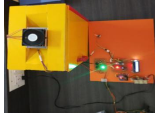
Fig. 9 Experimental Setup of Refrigerator, Buck Converter Arduino Nano etc.
