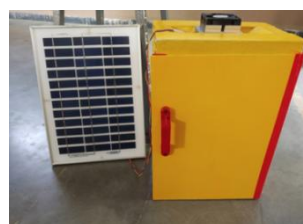
Fig. 8 Experimental Setup of Solar Panel and Peltier module.
