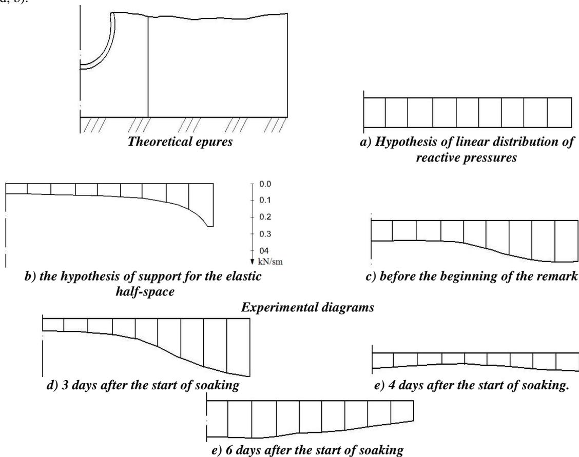
**Fig. 1. Plots of soil reactive force on the pressure from the diaphragm.**
