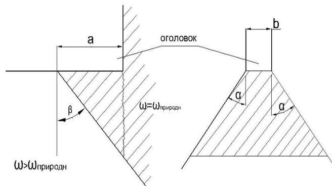
**Fig. 5. Diagram of the support of the tip-diaphragm on the wet ground wedge.**
