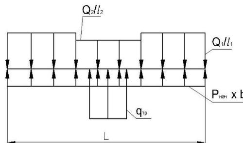
**Fig. 2. Design diagram of the diaphragm, corresponding to the case of its hanging on the water supply pipe.**
