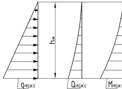
**Fig. 7. Design scheme of the work of the diaphragm from the pile of soil on the side of the water supply pipe.**
