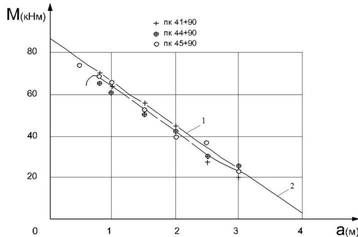
Fig. 6. Graphs of the change of the maximum bending moment in the tip of the crossing-differential depending on the parameter "a": 1- by the formula (8); 2- according to experimental data.
