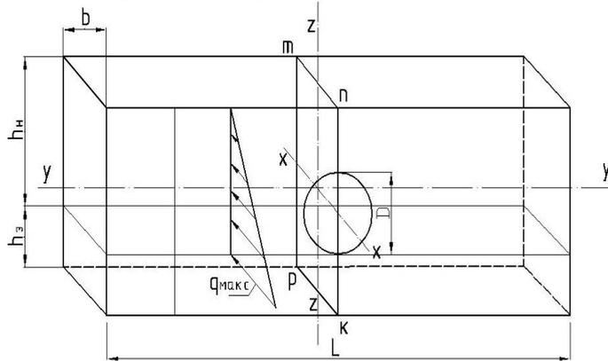
**Fig. 8. Diagram of the head-end diaphragm**
