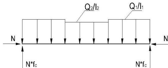
**Fig. 9. Design diagram of the diaphragm for the case of pile of soil on its side faces.**
