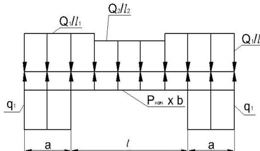
**Fig. 4. Design diagram of the diaphragm corresponding to the case of a partially moistened soil.**
