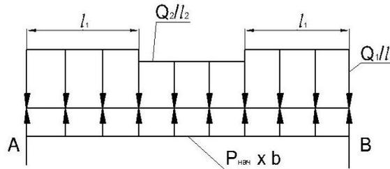
**Fig. 3. Design diagram of the diaphragm, corresponding to the case of the support of its edges on non-humid soil.**
