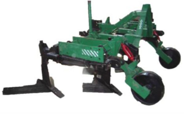
Fig. 1. Universal vineyard machine UUM-3 in the assembly version for the cultivation of rows and inter-creep stripes in vineyards with a row spacing of 3.0 m.
