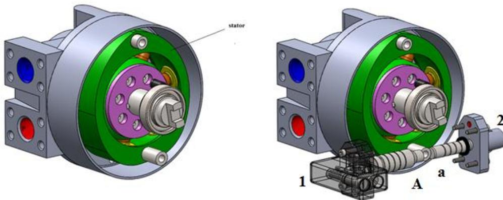
Figure 7: radial piston pump and actuators acting on its stator [4].
