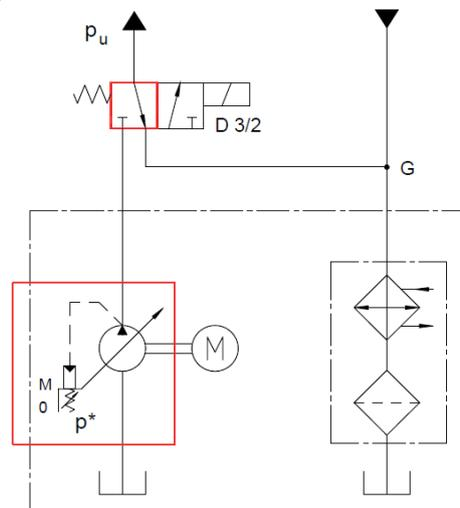
Figure 1. ISO scheme of direct acting absolute pressure limiter [3].
