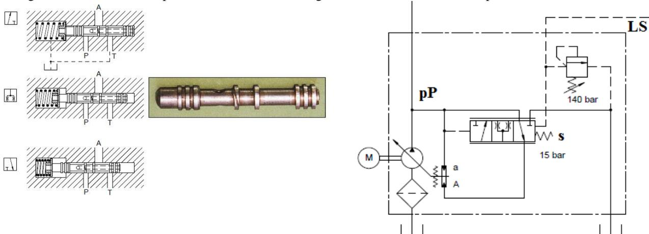
Figure 5: On the left, spool of the valve and on the right ISO scheme of differential pressure limiter given in [3].
