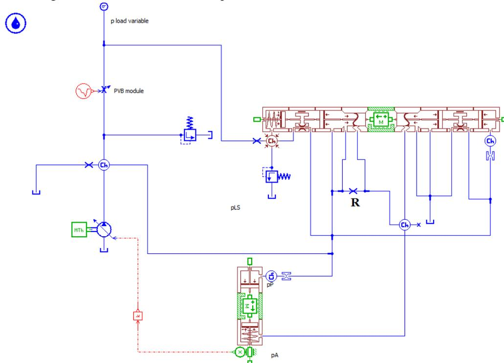
Fig 10: Amesim model of the differential pressure limiter
