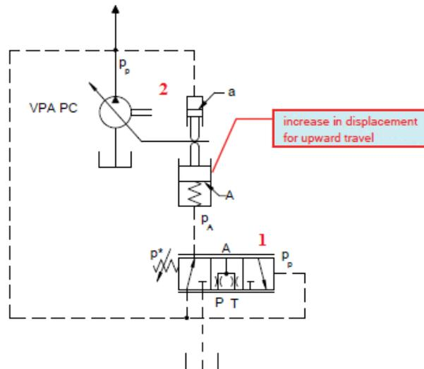
Figure 4: ISO scheme of a piloted absolute pressure limiter [3].
