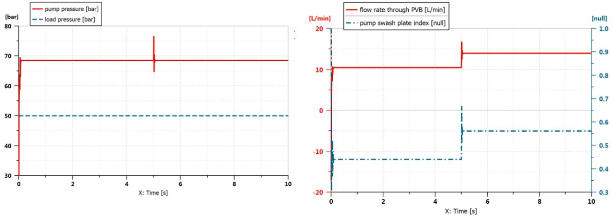
Figure 11. Pump pressure remains constant while orifice signals change (left figure). On the right, flow rate through PVB increase (solid line) as a consequence of pump swash plate index increase (dotted line).
