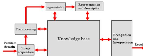
**Fig.6. Fundamental Block Diagram of Image Processing**
