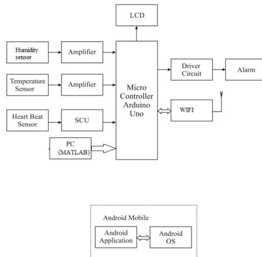
**Fig.3. Block diagram of Neonate Monitoring System****V. BLOCK DIAGRAM DESCRIPTION****A. ARDUINO UNO:**
