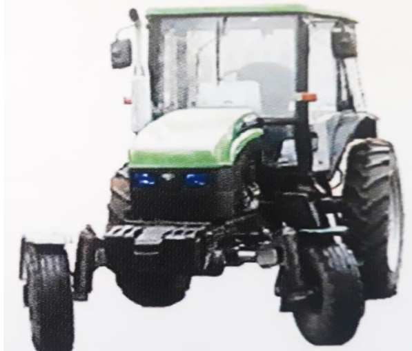
Figure 11: Experimental four-wheel tractor with increased passability and stability for desert zones, based on TTZ
