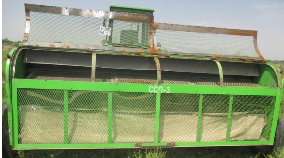
Figure 10: Experimental mower for harvesting hay and collecting seeds of arid fodder plants, SSP-3, rear view
