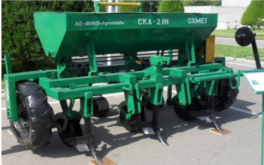
Figure 7: Experimental mounted seeder SKA-2,1N for sowing seeds of arid fodder crops (in particular, creation of seed plants)
