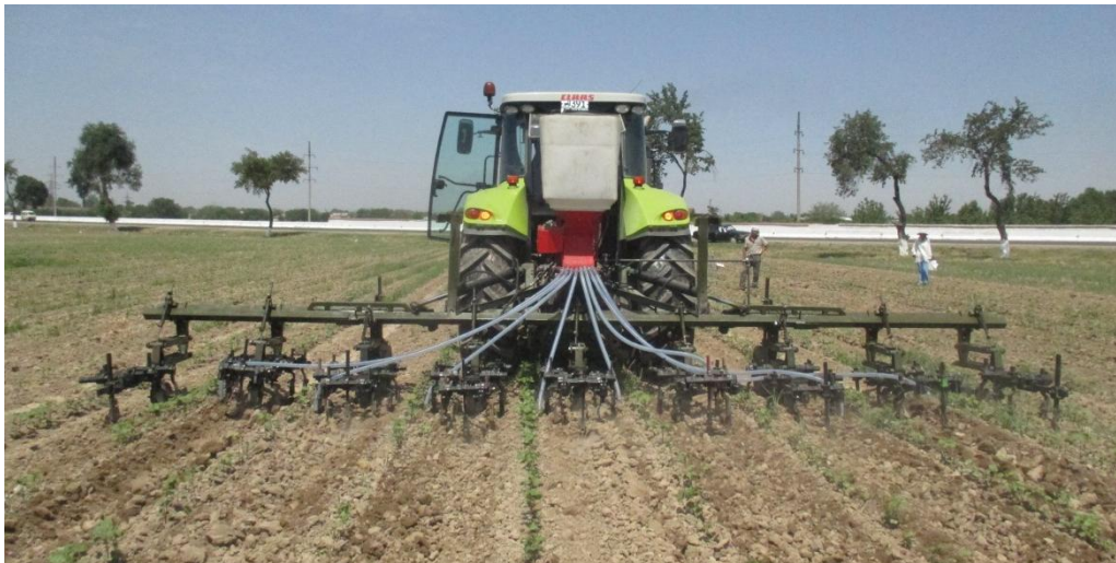
Figure 2. Experimental 8-row cultivator (conditionally KXY-8e) on cotton cultivation, 04.23.2019 at test site of the Center
