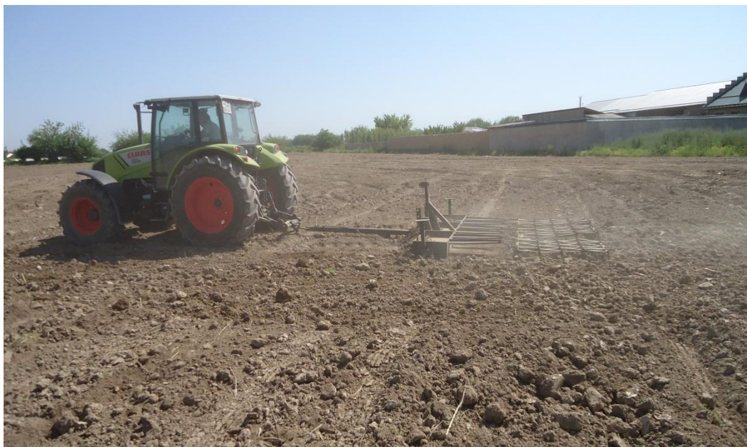
Figure 1. Experimental small-leveler MT-3M in preparing the field for sowing cotton
