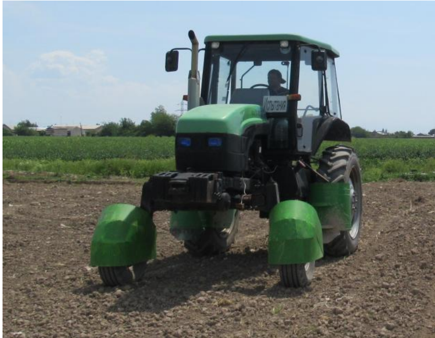
Figure 3. Experimental universal row-crop four-wheeled tractor equipped with a rear axle with stepless adjustment (in the field at factory test)
