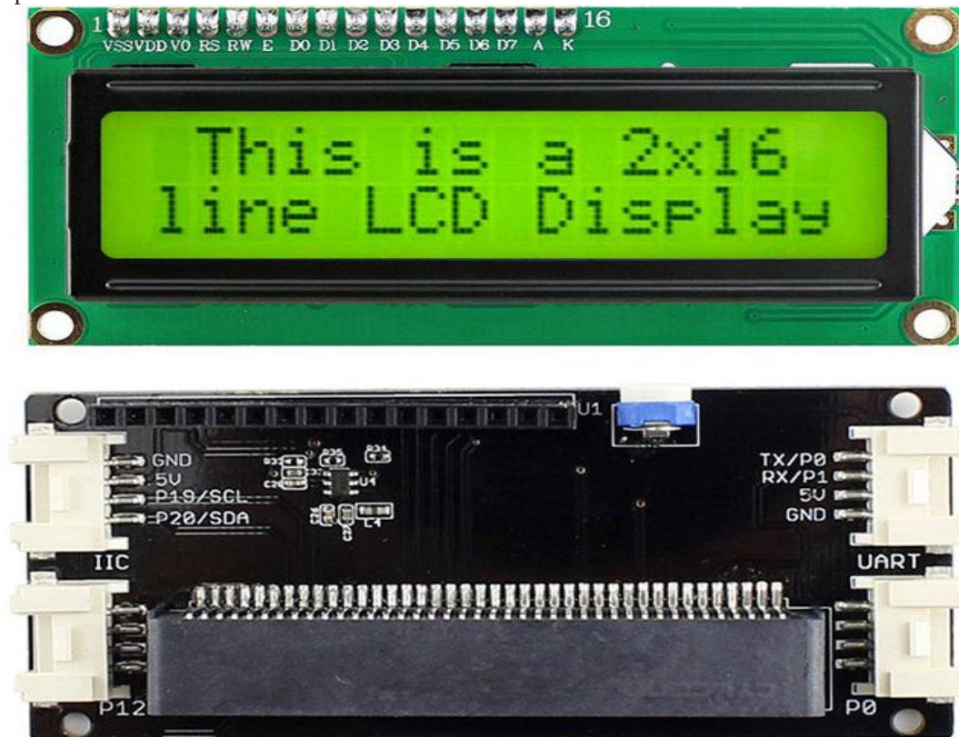
Figure 1. The front and back of the LCD1602 labeled device photo from the back
