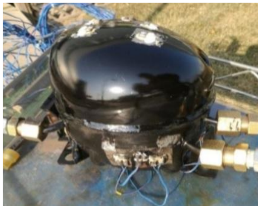
Fig1. Thermocouples mounted on the shell
