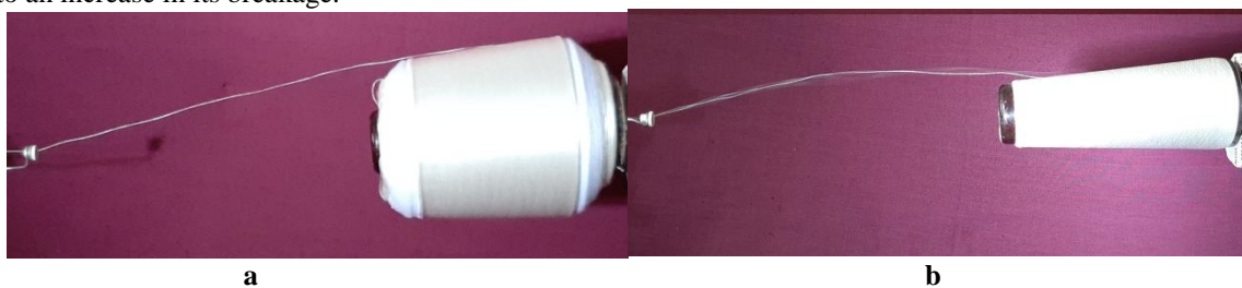
Fig. 3. Shapes of cylinders of silk thread at a winding speed of 200 m / min
