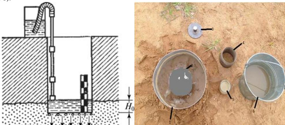
**Fig. 1. Installation diagram for determination of filtration coefficient by A.K. Boldyrev method**
