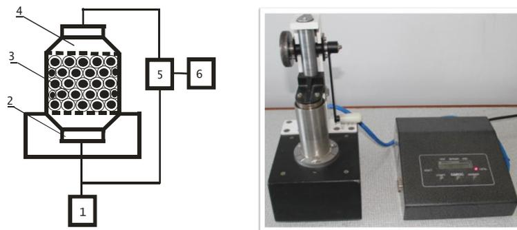
Figure 1 –Block diagram and overview of residual lint acoustic measuring instrument.
