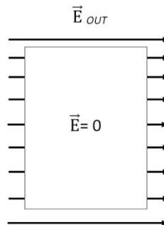
Fig. 1. Electrostatic field of conductors.
