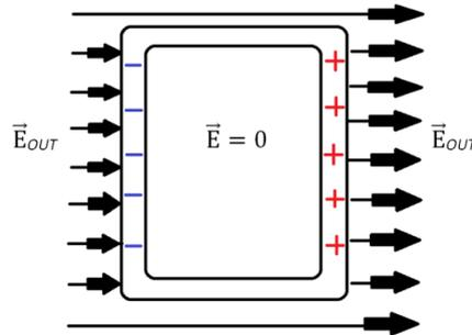
Fig.3. Electrostatic shield
