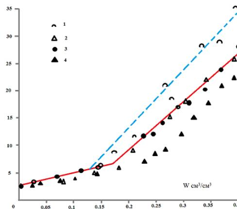
Fig. 9. Dependence of the real part of the CDC on the volumetric moisture: 1.2 - humus content 0.6%; 3.4 - with the addition of 30% ash; 1.3 - frequency 0.25 GHz; 2.4 - frequency 4.5 GHz (the lines show the approximation of the data of both samples at a frequency of 0.25 GHz).
