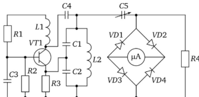
Fig. 7. Scheme of dielectric moisture meter.
