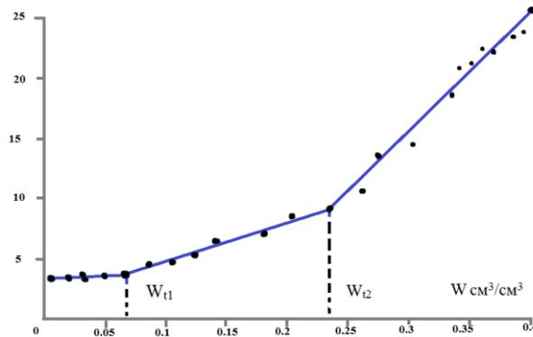
Fig. 8. dependences of the real part of the CDC of sample V1 (humus content 6.6%) on the volume humidity with the release of a section of strongly bound water (humidity  $W < W_{t1}$ ), loosely bound water (humidity  $W_{t1} < W < W_{t2}$ ) and free water ( $W > W_{t2}$ ) at a frequency of 4.5 GHz.
