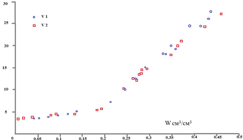
Figure: 10. Dependences of the real part of the CDC on the volumetric moisture content of samples V1 (humus content 6.6%), V2 (with the addition of ash 30% by mass to V1) at a frequency of 4.5 GHz.
