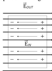
Fig.2 Electrostatic induction
