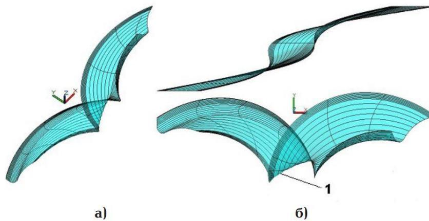
3-picture.Screw model of the surface (a) and its orthogonal projection (b); 1-Surface discriminant (the deflector part of the profile)
