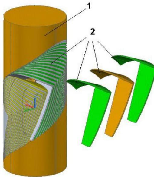
6-picture. After the formation of the detail Model (1) and the deleted layers (2)
