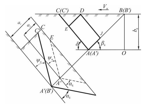
Scheme of impact of oblique wedge of AES on soil formation: AC-wall of open furrow; Case ploughshare AV-edge
