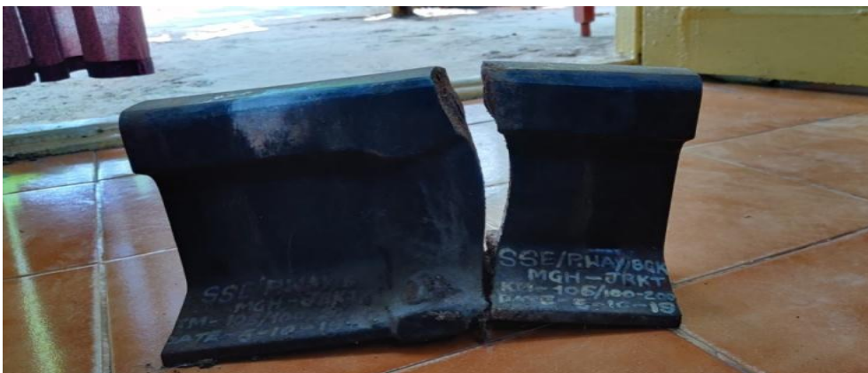
Fig 2.1: crack above 32mm
