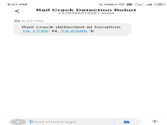
Fig 5.2: Location of crack detected sent through message
