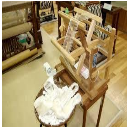
Figure 2. Mechanical machine for rewinding silk at home
