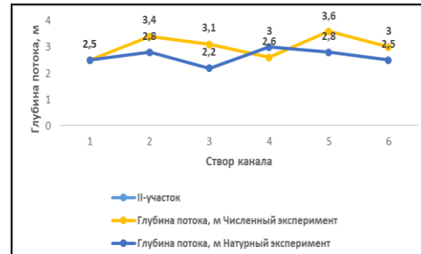
Fig. 5. Changes in water level in the II-section of the canal
