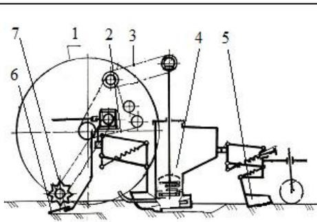
Fig. 1. Diagram of a cotton seeder equipped with a soil sweeping device. 1-frame; 2-wheel; 3-drive device; 4- sowing section; 5- sealing section; 6 ploughshare; 7-block loosening stars.
