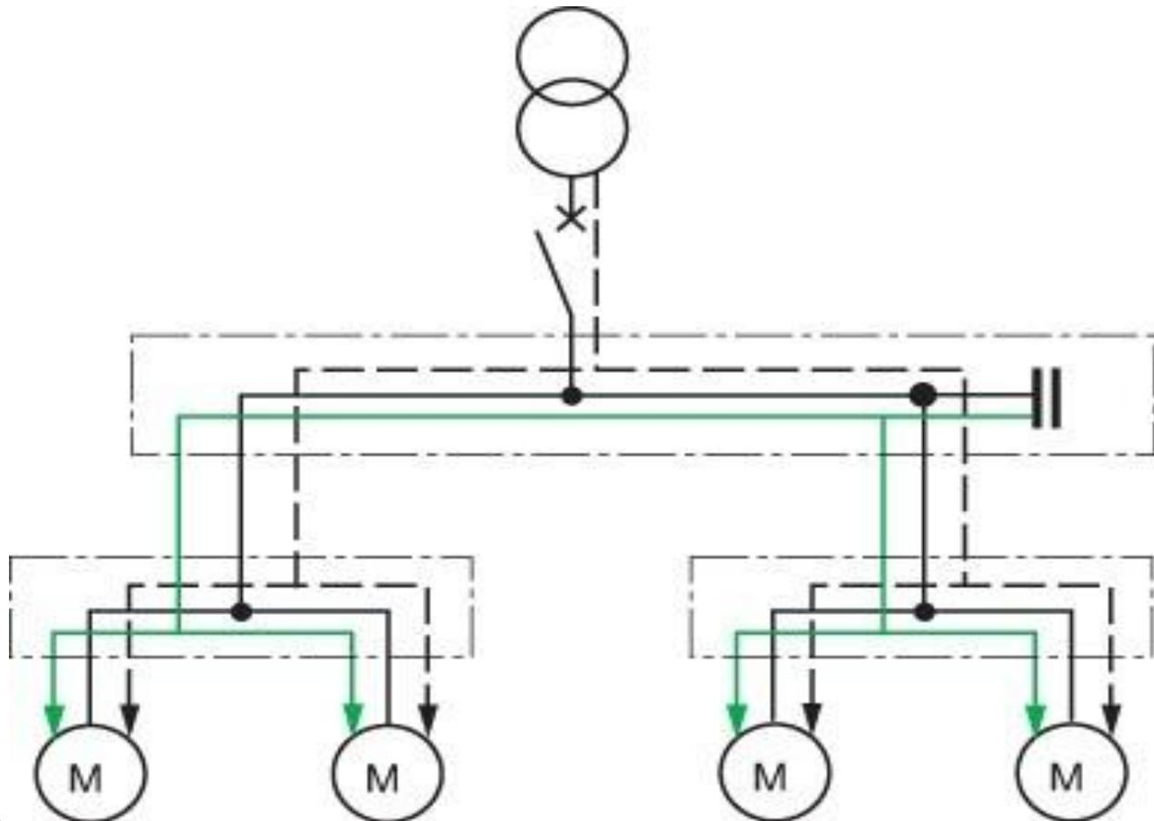
**Fig. 2. Scheme of centralized compensation of the reactive component of power consumption**
