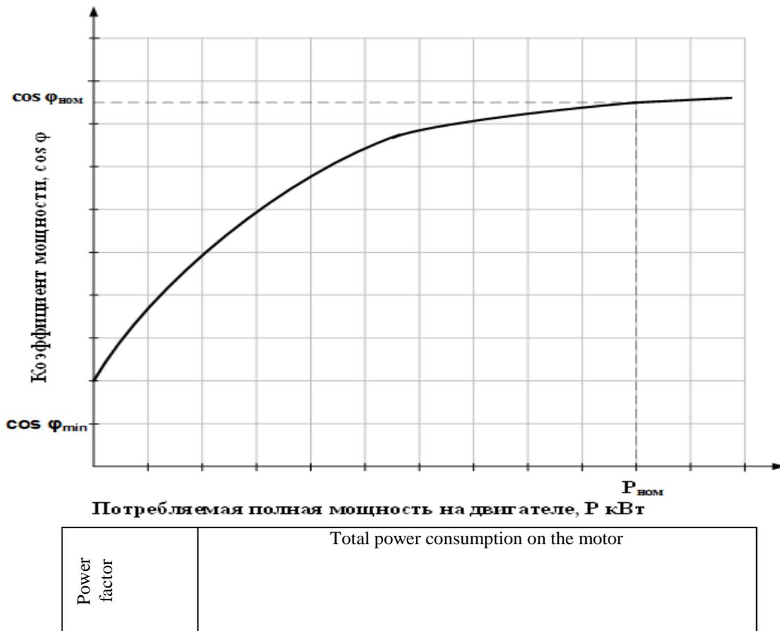
**Fig.1 Diagram of power factor dependence on motor load**
