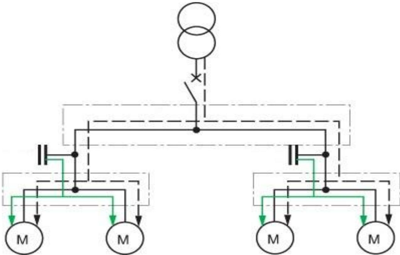
**Fig. 3. Scheme of sectional compensation of the reactive component of power consumption**
