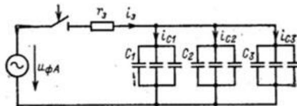
Fig. 2. Scheme for calculating zero sequence currents during transients.
