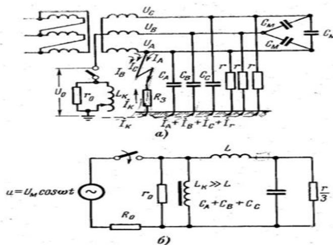
Fig. 1. Equivalent circuits of a network operating with isolated neutral and with compensation of capacitive currents. a - three-phase; b - zero sequence.
