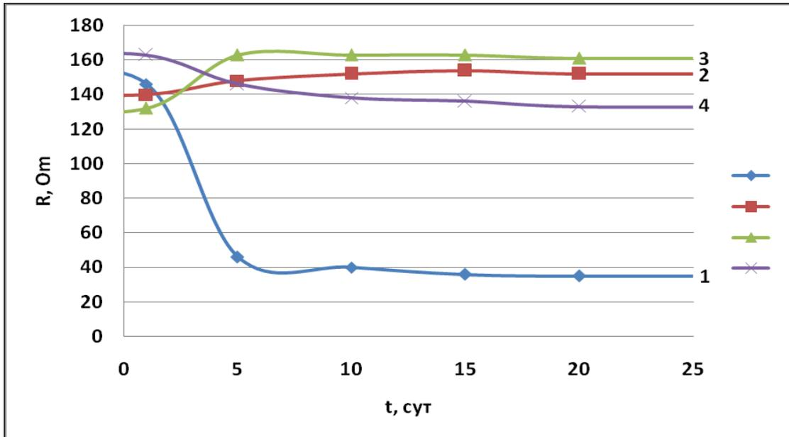
Figure-2. The dependence of the polarization resistance on time in a solution of 3% H2SO4 in the presence of a coating.
