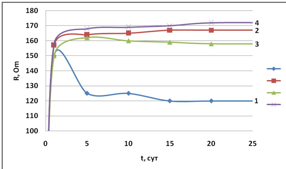
**Figure. 1. Dependence of polymerization resistance on time in 3% NaCl in the presence of a coating:**
