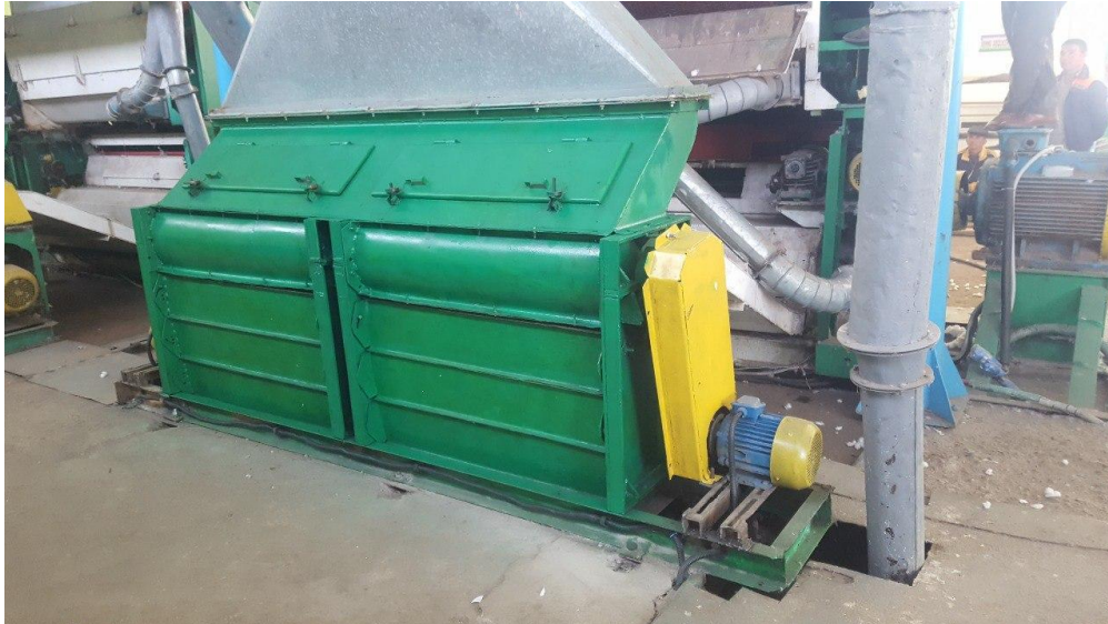
Figure 3. General view of the fiber cleaner, modernized and installed at the plant
