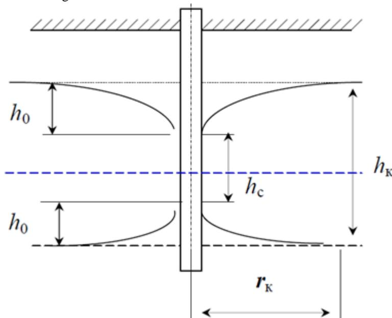
Fig. 1 Scheme of the formation of gas and water cones
