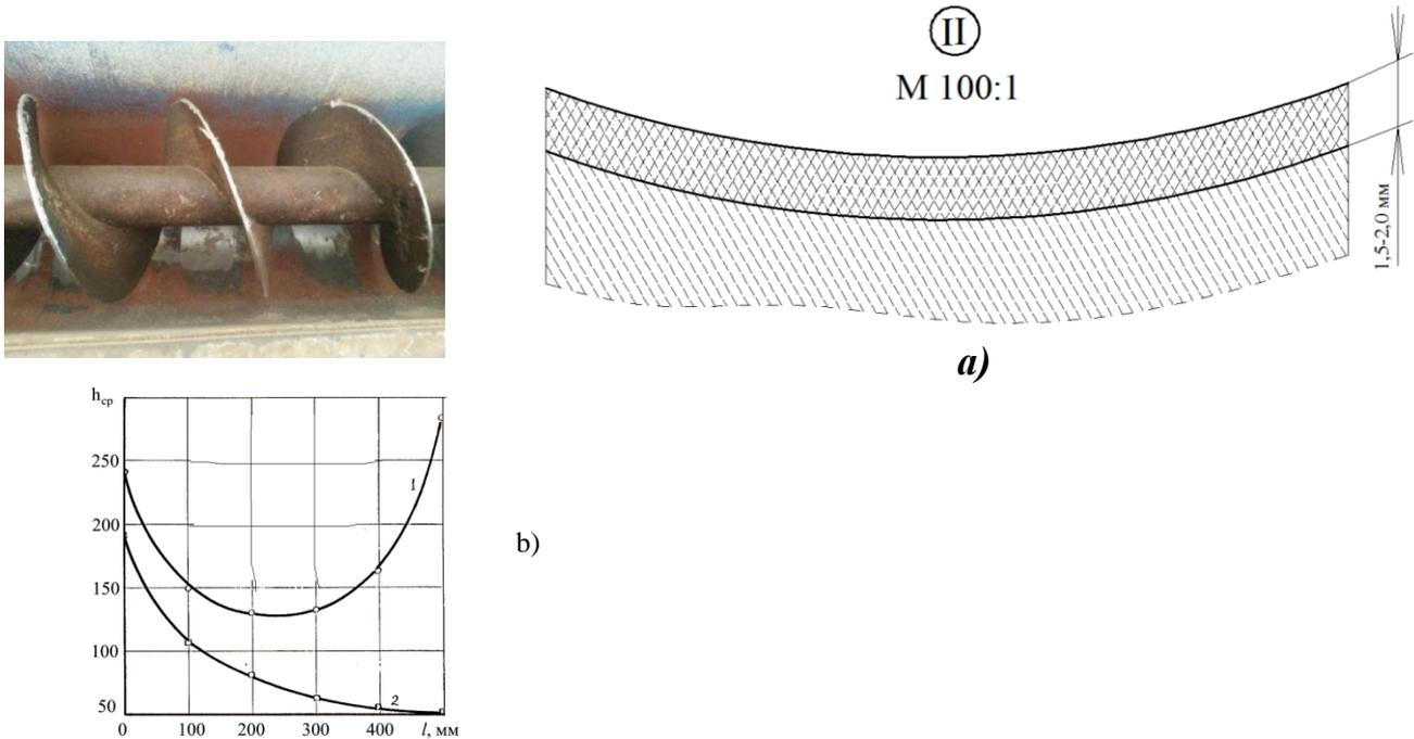
Figure 2. Scheme of obtaining multifunctional coatings containing GKP material -1,2,3 in cotton screw conveyor (distributor) screw and jellies (a) and their service life forecasting schedule (b).
