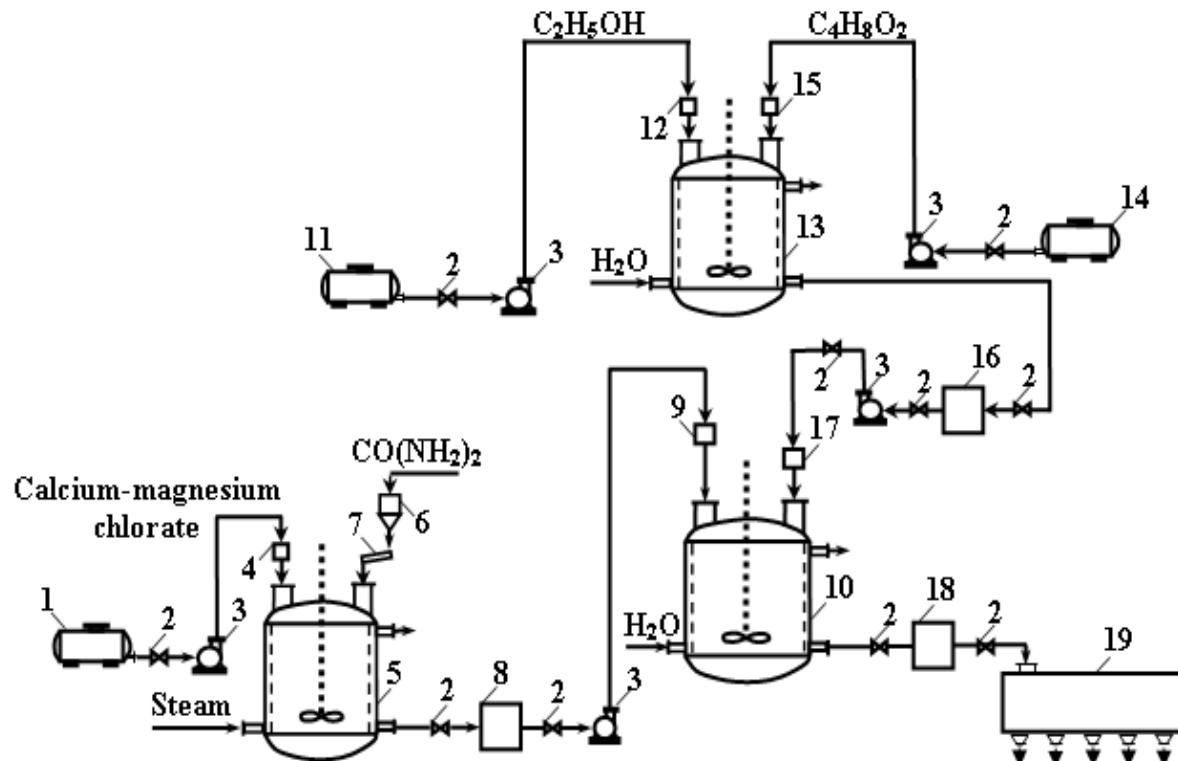
Figure 2. The basic technological scheme for obtaining of new defoliant
