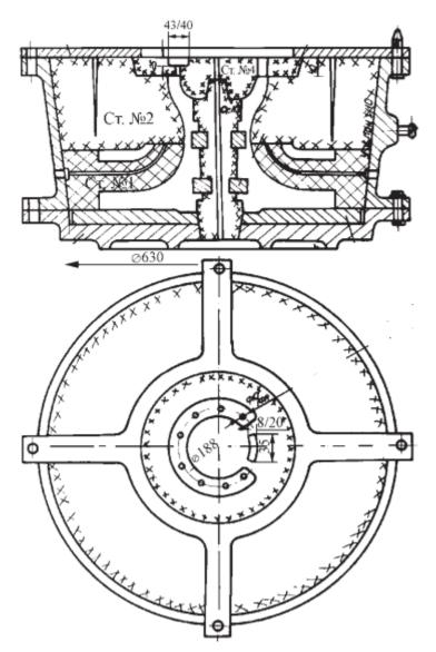
Figure: 6. Scheme of forming 8NP impellers using a refrigerator (insert)
