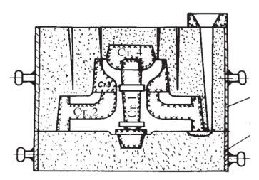
Figure: 5. Scheme of forming impellers 8NP
