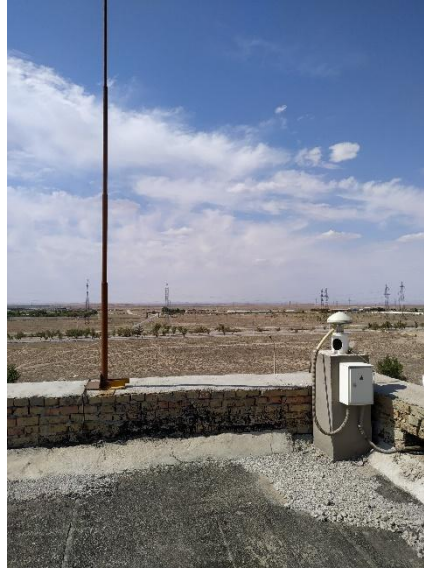
Figure 5. Permanent GNSS base station antenna (Zarafshan ZAR1)
