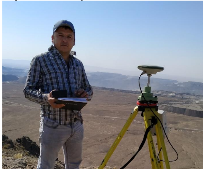
Figure 6. Geodetic survey process (Static method) with Leica GS10 GNSS receiver in the territory of Muruntau gold deposit belonging to NMMC.
