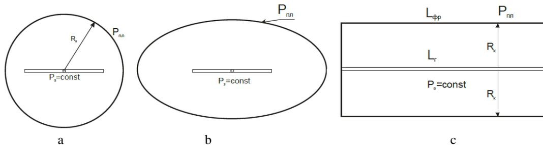
**Fig. 2. Diagrams of the drainage zone shapes for a horizontal well: a-circular (according to Borisov and Tabakov); b-ellipsoidal (according to Giger, Saadi S. Joshi); in-rectangular (proposed by Z.S. Aliev)**
