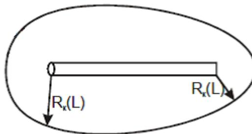
**Fig. 3. The shape of the zone of the drained horizontal well, taking into account the change in bottomhole pressure along the length of the horizontal section of the wellbore:  $R_k(L)$  - the radius of the feed loop as a function of the length of the horizontal section of the wellbore**
