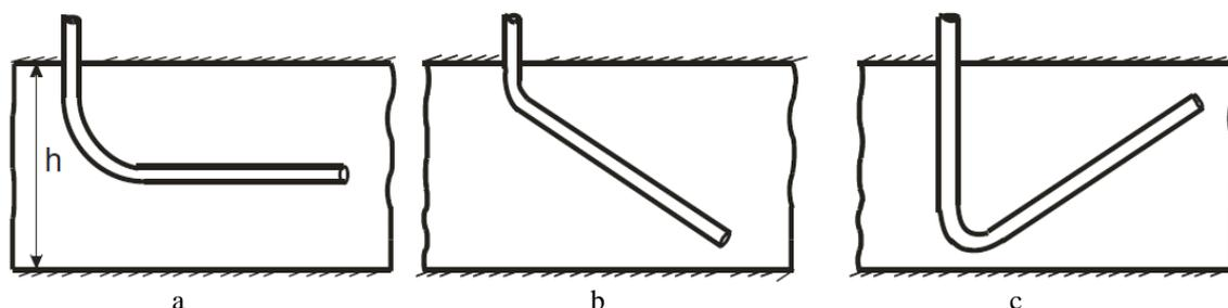
**Fig. 1. Opening schemes with a horizontal wellbore with different profiles: a - horizontal, b - descending with a single zenith angle, c - ascending with a single zenith angle**
