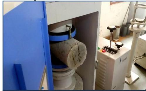
❖ **Data of Split Tensile strength of concrete**
