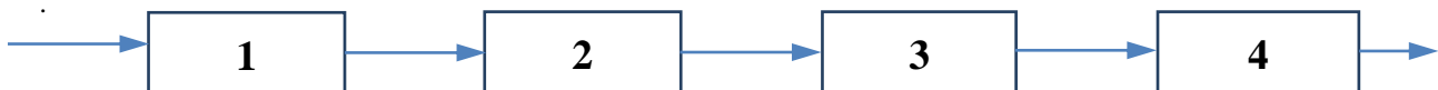
Fig. 6. Scheme of the experimental device for the study of thermoanemometric type heat exchangers: 1 – thermoanemometric type heat exchanger; 2-RS-ZA type rotameter; 3 GSB 400 gas meter; 4 consumption motor (pump)
