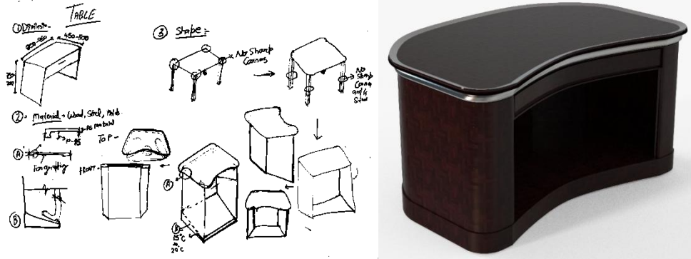
Fig3. Table Detail and Design as per discussion with dis-able person.
