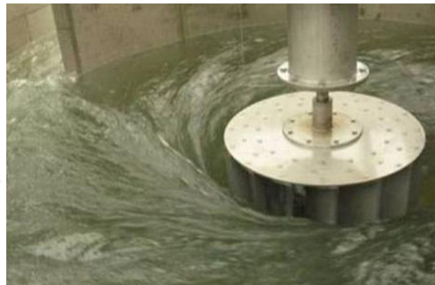
Fig.5. Gravitational vortex microhydroelectric power plant.
