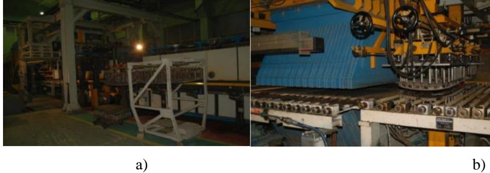
Fig. 3. Technological equipment - Continuous horizontal furnace a) Heating section b) Press and tempering section
