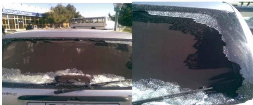
Fig. 1. Self-destruction of the automotive rear window glass.
