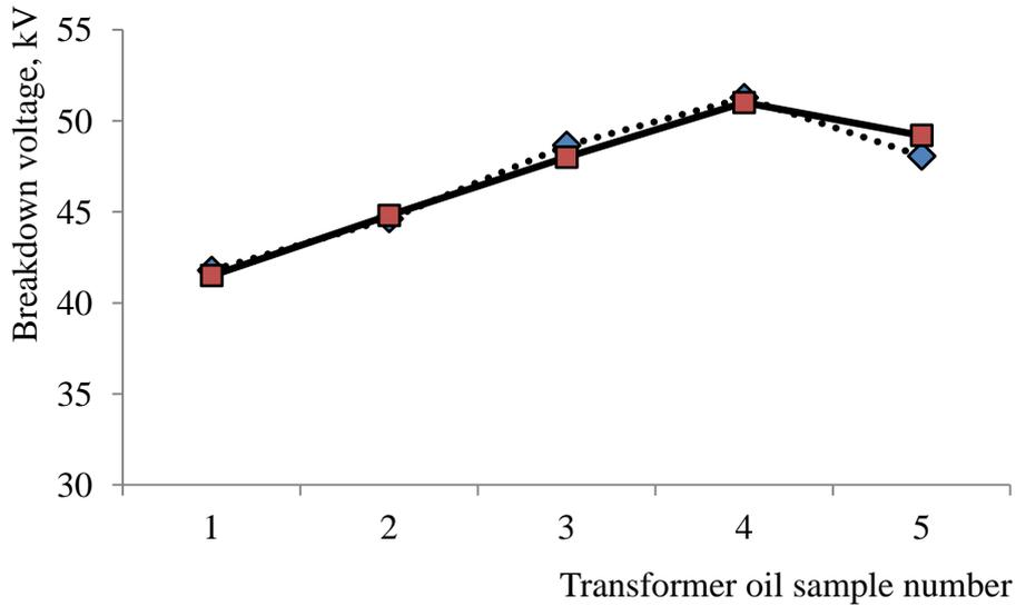
Fig.2. Experimental and calculated values of the breakdown voltage of the used transformer oil after cleaning with a ceramic membrane filter and an adsorbent (silica gel)
