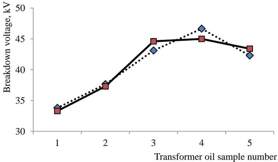
Fig.1. Experimental and calculated values of the breakdown voltage of the used transformer oil after cleaning with a ceramic membrane filter
