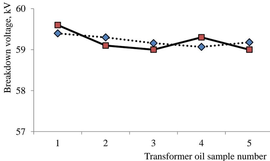
Fig.3. Experimental and calculated values of the breakdown voltage of the used transformer oil after cleaning with a ceramic membrane filter and adsorbents (silica gel and zeolite)
