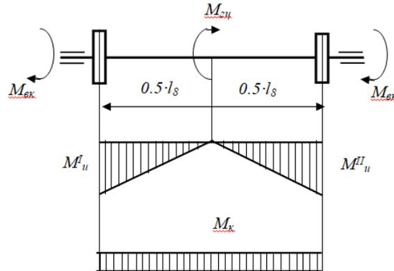
Fig 1. Diagram of bending and torque moments of the rocker shaft
