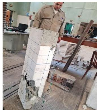
**Fig.9: Failure mode for column H0.5, 1.5.**
