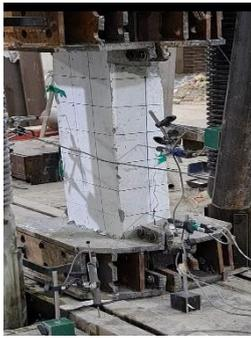
**Fig.6: LVDTs setup.**
