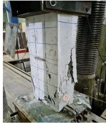
Fig.10: Failure mode for column H1,1.5.
