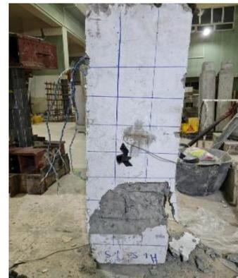
Fig.11: Failure mode for column H1.5,1.5.
