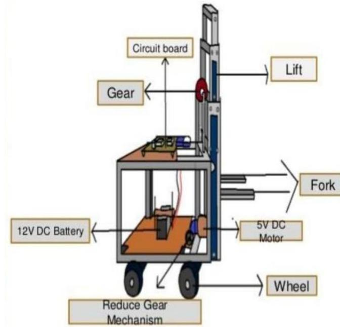
**Fig. 3.1. Forklift material handling system**
