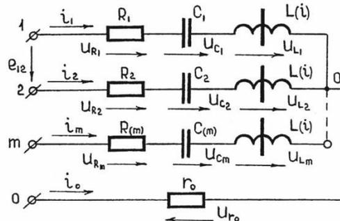
Figure 3. Multi-phase ferroresonant circuit with zero conductor and no ferro-magnetic coupling between the non-linear coils.
