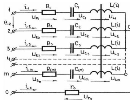
Figure 5. Multi-phase ferroresonant circuit with zero conductor c ferromagnetic coupling between the non-linear coils.
