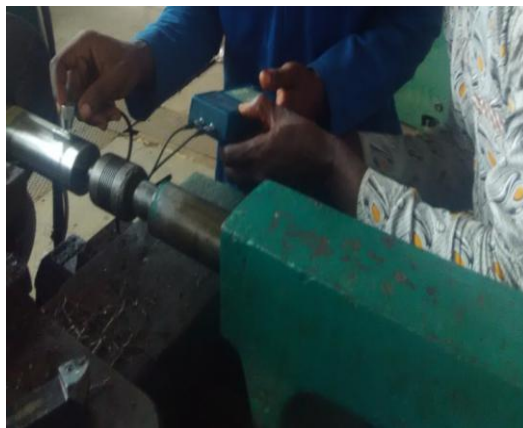
Plate 3: Measuring and reading roughness value
