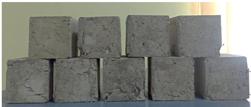
Figure 3. General view of cube-samples made of non-basalt fiber concrete (a) and basalt fiber concrete (b)
