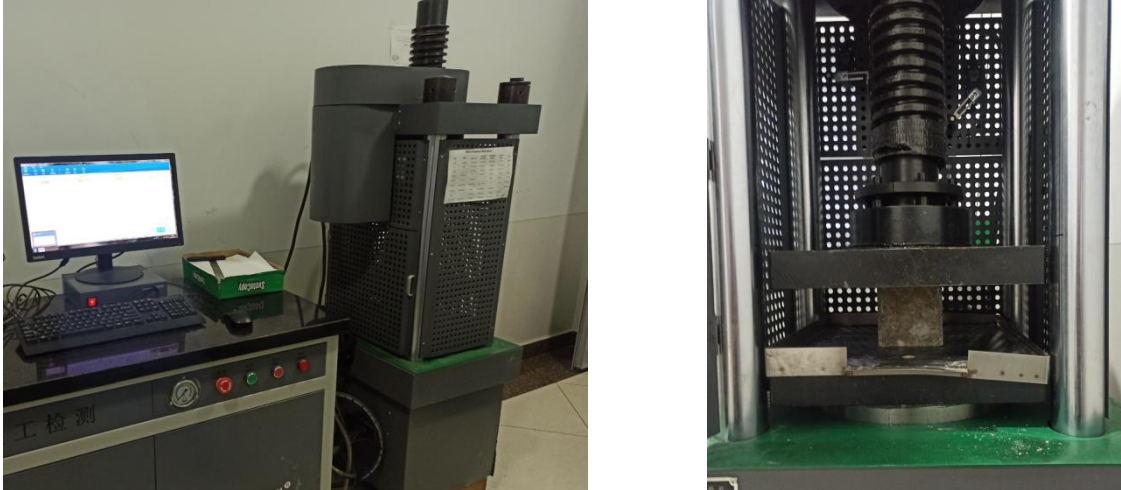
Figure 2. General view of the test device and the cube-sample.
