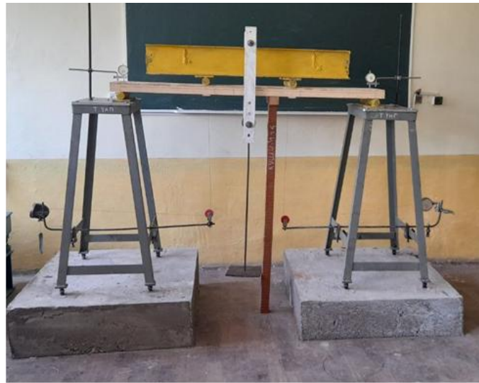
Figure 2. Lightweight wooden roofing slab before loading.
