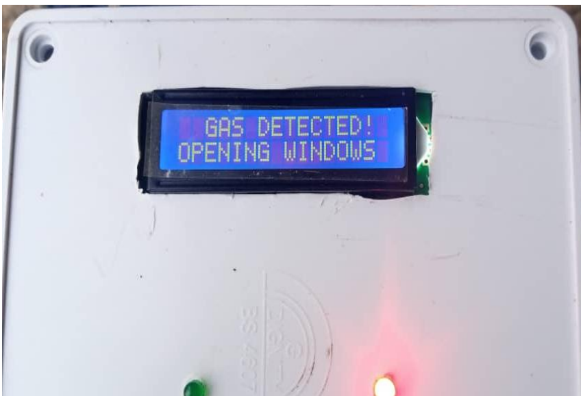
Figure 5: interface showing Gas leakage detected opening window
