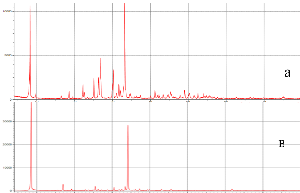
Fig. 2. X-ray phase analysis of monochloroacetic acid sodium (a) and double aqueous monochloroacetic hydroxycalcium (b).
