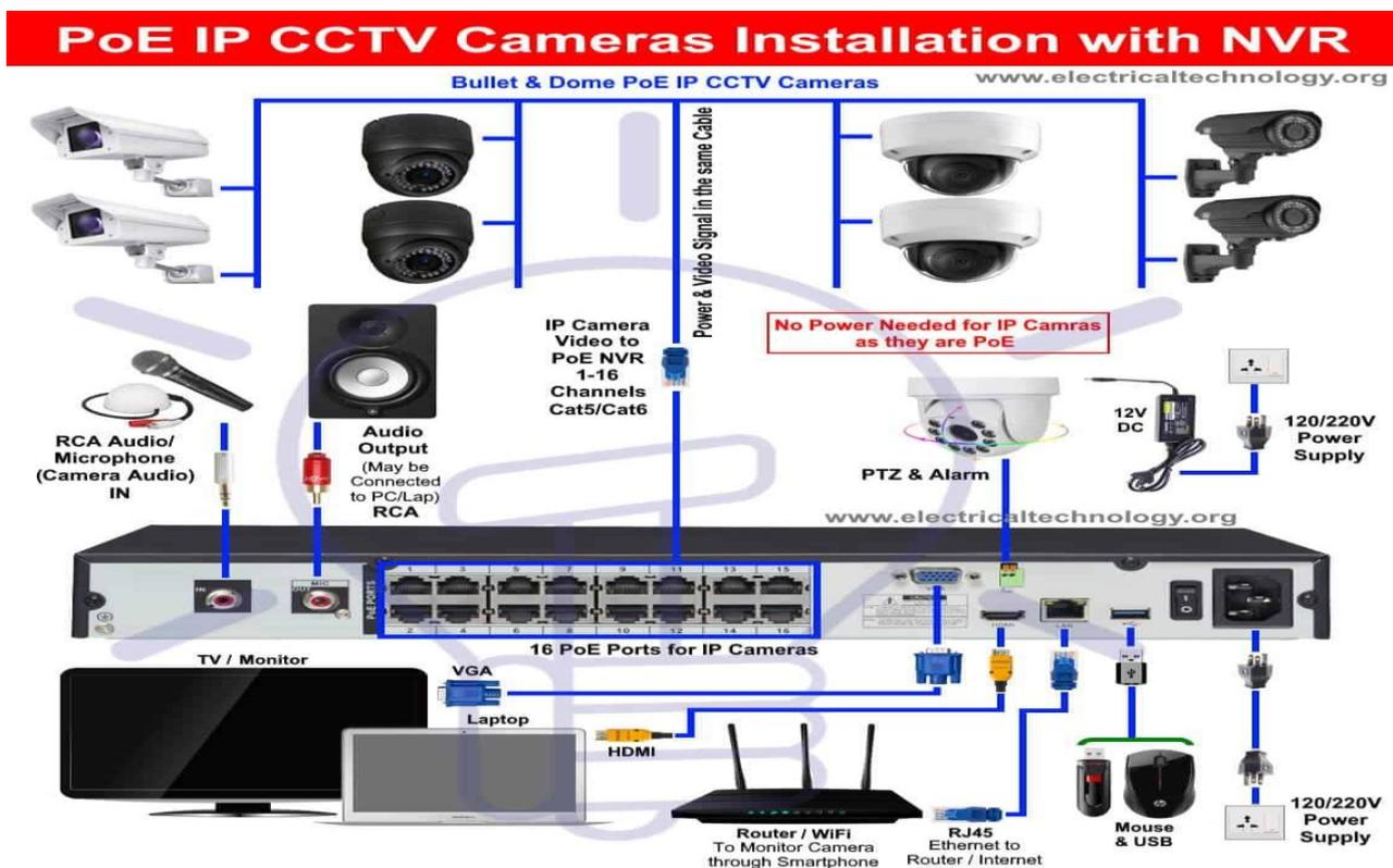
Figure 7: PoE IP CCTV cameras security system with NVR. [20]
