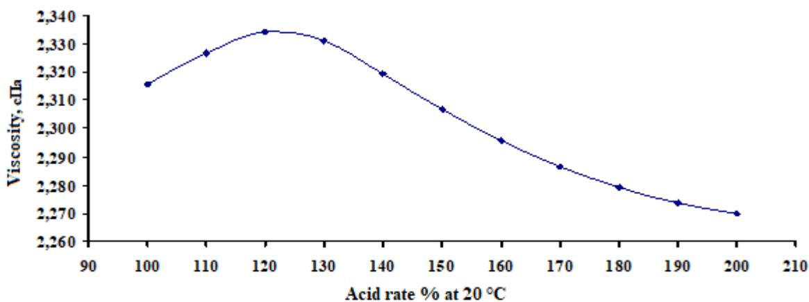
Fig. 4. Change in the viscosity of the liquid phase depending on the rate of nitric acid at a measurement temperature of 20°C
