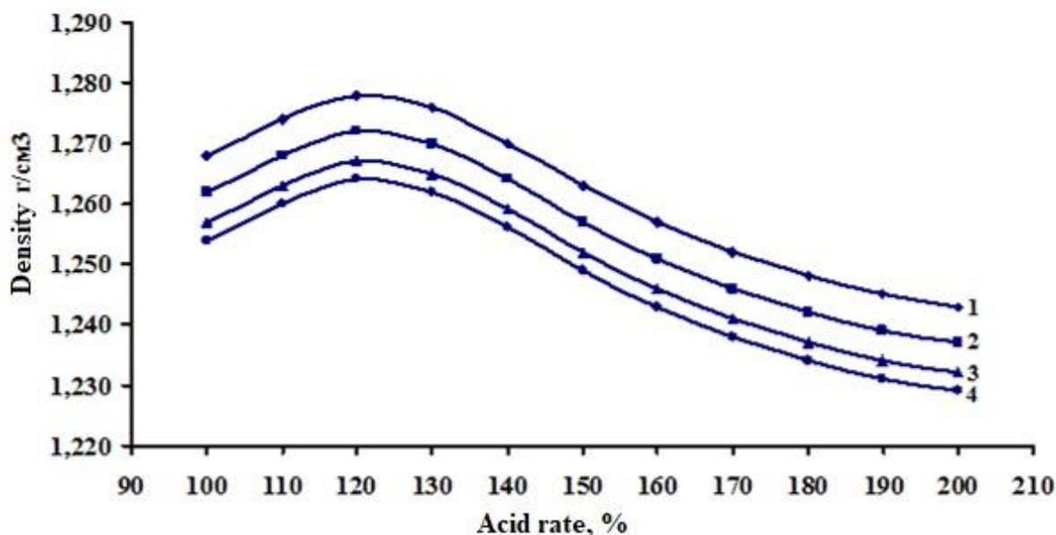
Fig. 3. Change in the density of the liquid phase depending on the norm of nitric acid at the measurement temperature of 1-20°C, 2-40°C, 3-60°C and 4-80°C.
