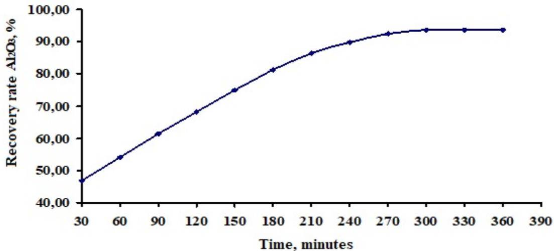
Fig. 1. Influence of the duration of the leaching process on the degree of extraction of aluminum at a temperature of 150°C, a concentration of nitric acid of 30% and a norm of 130%
