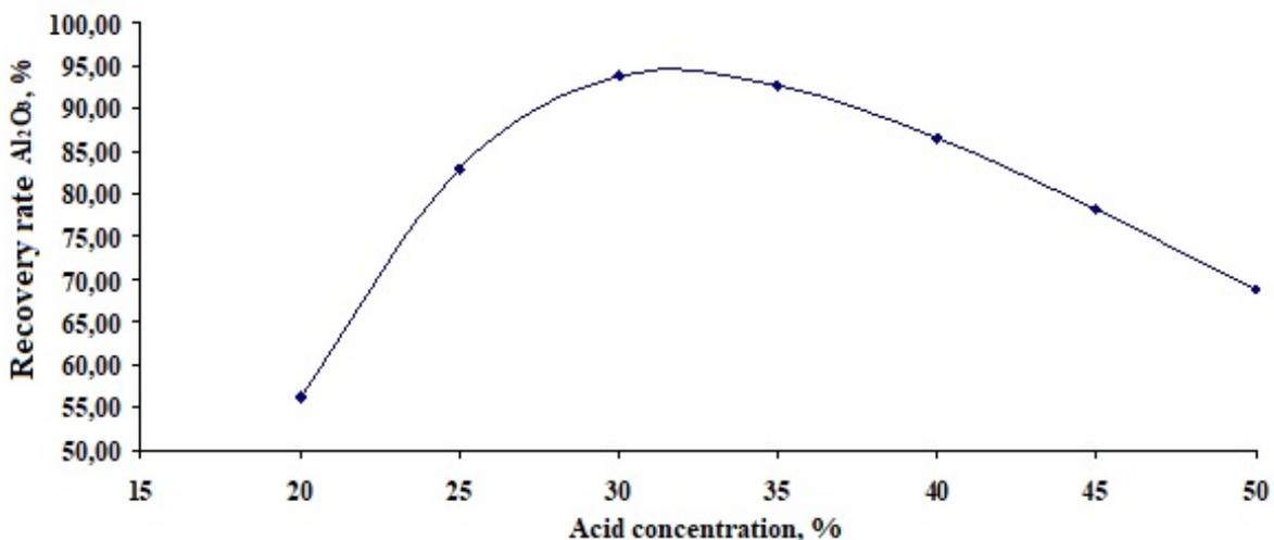
Fig. 2. The effect of nitric acid concentration on the degree of aluminum extraction at an acid rate of 130%, a temperature of 150°C and a process duration of 5 hours
